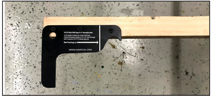
Wheel profile gauge attached to 2X2
